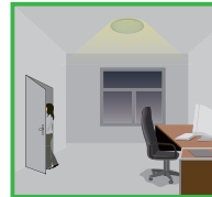
People left, light still dims to 0/ 10%/20%/30% if with insufficient ambient light.
