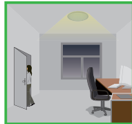
People left, light dims to 0/ 10%/20%/30% (options) standby level after the hold time.
