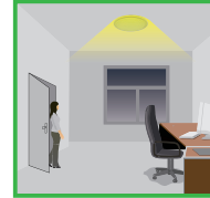
With insufficient natural light, the sensor switches 100% on the light automatically when person enters the room.
