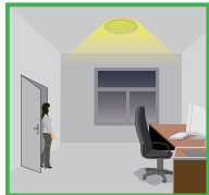
With insufficient ambient light, the sensor switches 100% on the light automatically when person enters the room.
